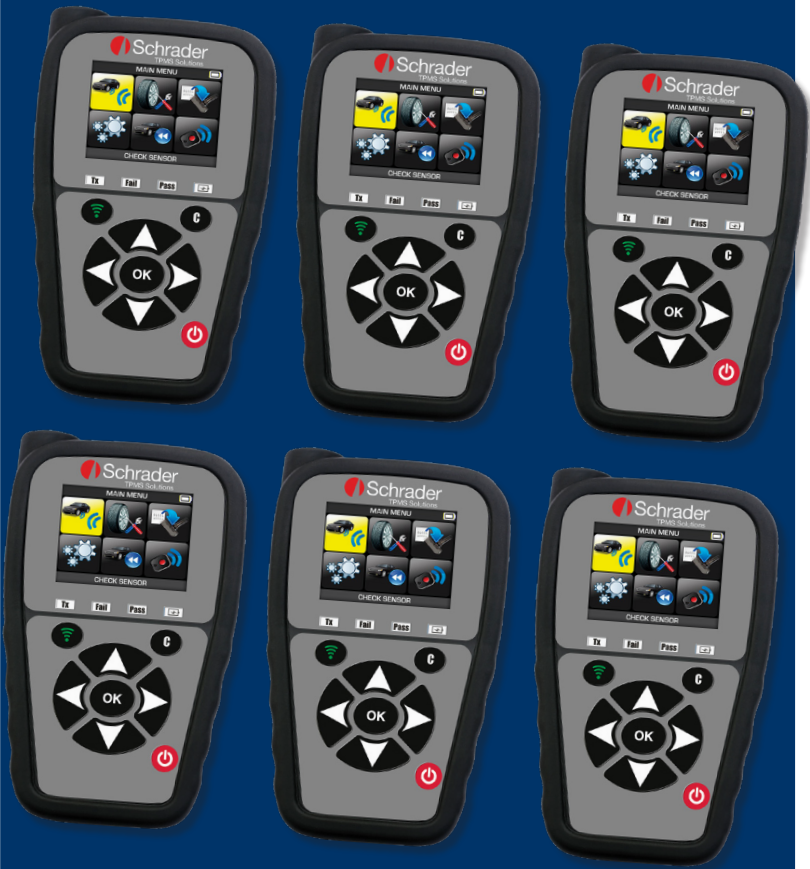
Six S41 TPMS Programming and Diagnostic tools
